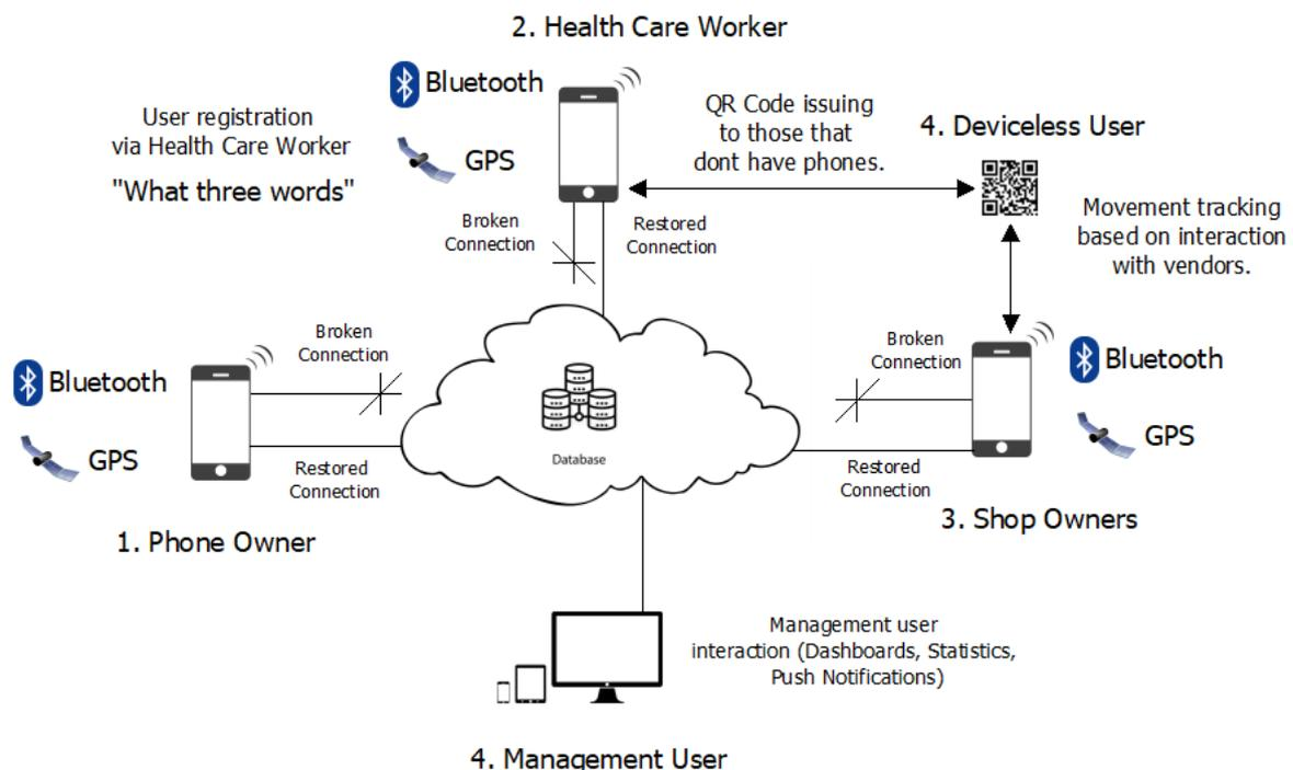
Figure 1: High level functional view of the solution.
